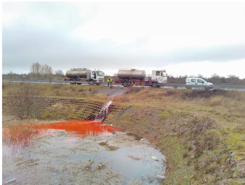
Photo 3 – injection, le 24/11/2016, de 16 kg de sulforhodamine B
