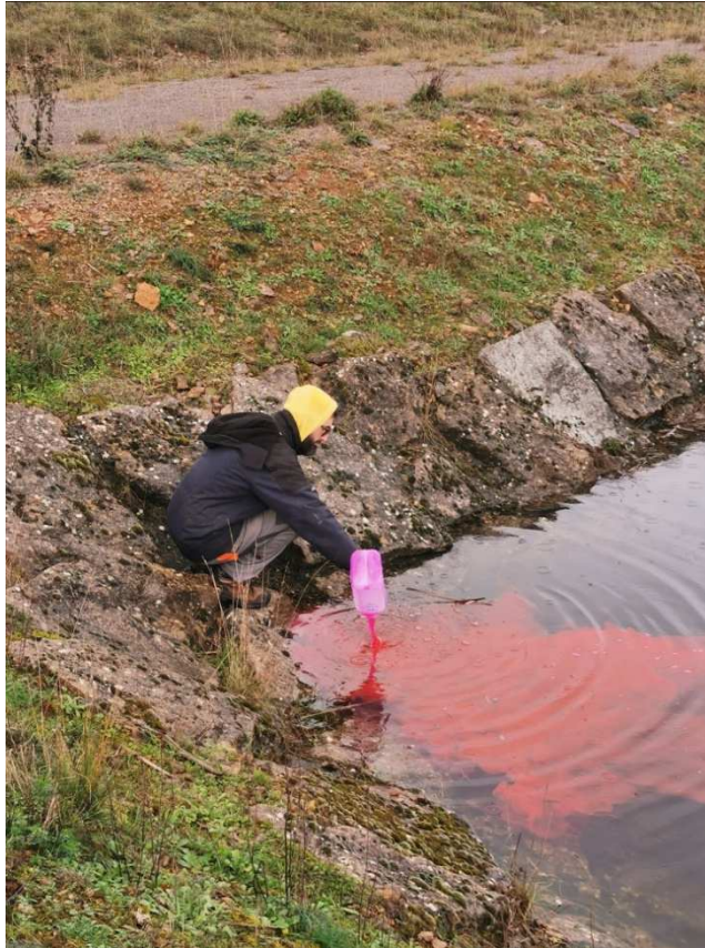
Figure 7 – injection, le 23/11/2022, de 400 g de sulforhodamine B
